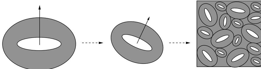
**Fig. 4.** Assemblage of self-similar randomly oriented hollow ellipsoids. Unit pattern (left). Rotated and dilated hollow ellipsoid (center). Representative volume element (right).
