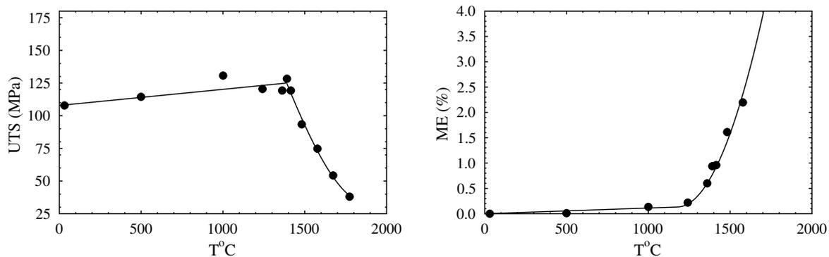
Fig. 2. Ultimate tensile stress (UTS) and maximal elongation (ME) versus temperature for non-irradiated  $\text{UO}_2$  with 3% of initial porosity and 8  $\mu\text{m}$  grain size (after Canon et al., 1971).
