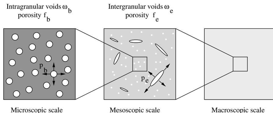
Fig. 3. Up-scaling (or homogenization) procedure.
