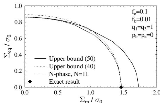
Fig. 5. Spherical voids in a Gurson matrix.  $f_e = 0.1, f_b = 0.01, q_3 = q_1 = 1$ . Drained case ( $p_b = p_e = 0$ ). Comparison between different predictions: upper bound (40) (dotted line), upper bound (50) (solid line), N-phase model ( $N = 11$ , dashed line), exact result (D.7) for hydrostatic loading (diamond).
