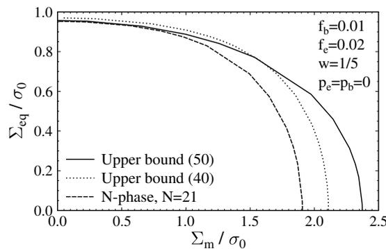
Fig. 11. Gurson matrix containing randomly oriented ellipsoidal voids.  $f_e = 0.02$ ,  $f_b = 0.01$ ,  $q_3 = q_1 = 1$ ,  $w = 1/5$ . Drained case ( $p_b = p_e = 0$ ). Comparison between different predictions: upper bound (40) (dotted line), upper bound (50) (solid line),  $N$ -phase estimate ( $N = 21$ , dashed line).
