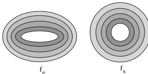
**Fig. 10.** “Equivalent porosities”: the effective elastic properties of the actual configuration (left, porosity  $f_e$ ) are identical to the effective properties of the virtual configuration with spherical voids (right, porosity  $f_s$ ).
