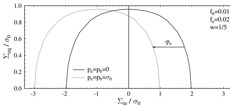
Fig. 15. Gurson matrix containing randomly oriented ellipsoidal voids  $f_e = 0.02$ ,  $f_b = 0.01$ ,  $q_3 = q_1 = 1$ ,  $w = 1/5$ . Estimate of the effective flow surface based on the  $N$ -phase model ( $N = 6$ ). Comparison between the drained case ( $p_b = p_e = 0$ , dashed line) and the saturated case with  $p_b = p_e = \sigma_0$  (solid line).
