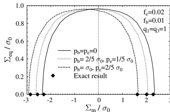
Fig. 7. Effective flow surface of porous materials containing two populations of spherical voids. Influence of the internal pressures on the effective yield surface.  $N$ -phase estimate ( $N = 6$ ),  $f_e = 0.02$ ,  $f_b = 0.01$ ,  $q_3 = q_1 = 1$ . Diamond: exact result (D.7). Drained case ( $p_b = p_e = 0$ ) and saturated cases:  $p_b = (2/5)\sigma_0$ ,  $p_e = (1/5)\sigma_0$ , and  $p_b = \sigma_0$ ,  $p_e = (2/5)\sigma_0$ .
