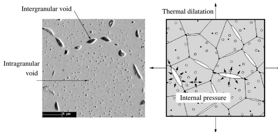
**Fig. 1.** (left) Micrograph of irradiated UO<sub>2</sub> (33 GW j/T) after heat treatment at 2000 K during 3 h (Dubourg et al., 2005). (right) Swelling of UO<sub>2</sub> during an accident. Development of thermal strains and internal pressures inside the cavities.
