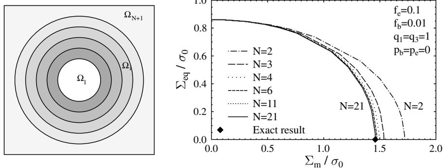
Fig. 6. (left) Multi-layered inclusion in an infinite matrix. (right) Influence of the number of subdomains on the accuracy of the  $N$ -phase model.  $f_e = 0.1$ ,  $f_b = 0.01$ ,  $q_3 = q_1 = 1$ . Drained case ( $p_b = p_e = 0$ ). Diamond: exact result (D.7).
