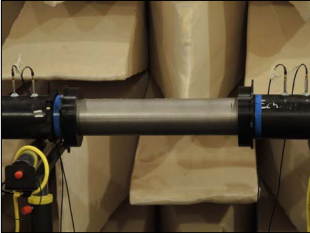
Figure 4. Close view of the two-microphones installed before and after the MPP section (without the annular duct).
