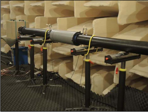
Figure 2. Photograph of the standing wave duct installed in the semi-anechoic chamber.
