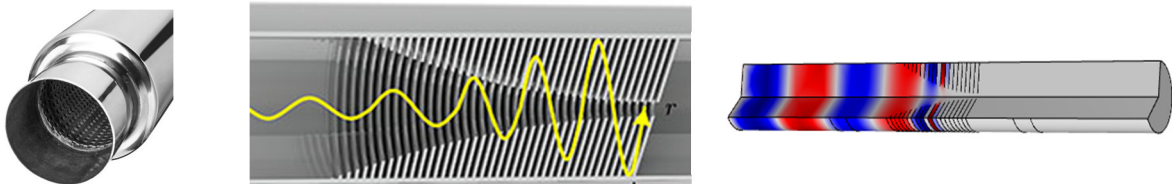
Figure 1 – (left) Perforated inlet of a typical exhaust muffler; (middle) schematic of a slightly open ABH (from Mi et al., Appl. Phys. Lett., 2021); (right) FEM simulation of the sound pressure field inside a slightly open ABH (from Bravo and Maury, 2021).
