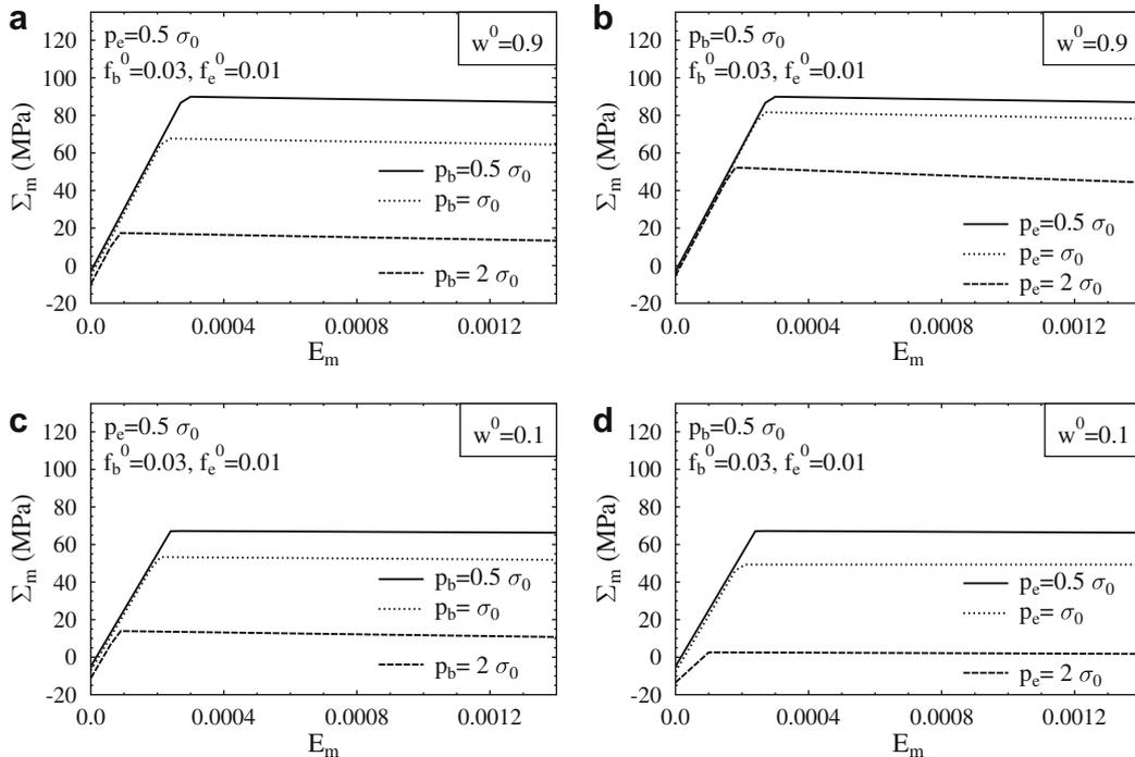
Fig. 4. Influence of the internal pressures  $p_b$  and  $p_e$  on the overall stress–strain response of a doubly voided material. Initial aspect ratio of the ellipsoidal cavities  $w^0 = 0.9, 0.2, 0.1$ .
